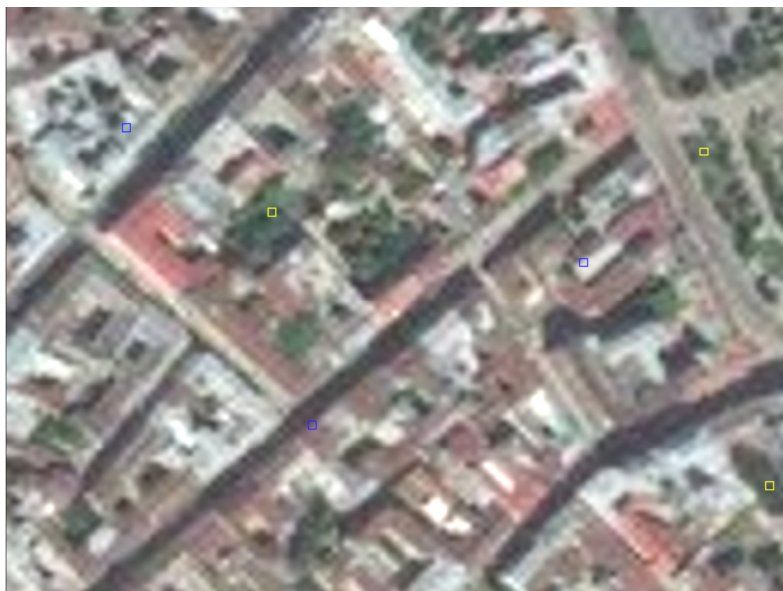
Fig. 9. Fragment of a satellite image of the city of Lviv with examples of determining the types of coverage: blue cells - improved waterproof surfaces; yellow cells - water-permeable surfaces
